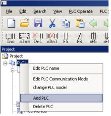
Method 2 : In project column which is on the left side, right-click "PLC1"—"Add PLC", as follows:
