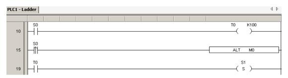
Click sDel (or press Shift+Del key), the row of dotted line box is deleted, the next row up will move a row automatically.
