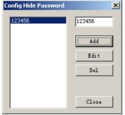
In the process of using a locked PLC frequently, or entering different passwords to different locked PLCs, the user can set a default decryption password. As shown above, the user can set a number of decryption passwords. Then during uploads there is no need to enter passwords repeatedly.
